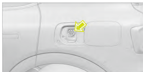
Location of discharging port of the vehicle.
